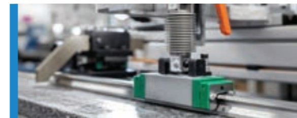
Cutting linear guides and assembling with carriages according to specifications.
