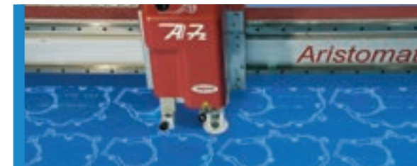
Production of flat seals from various materials.
