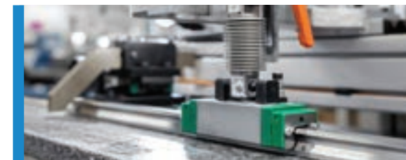
Cutting linear guides and assembling with carriages according to specifications.
